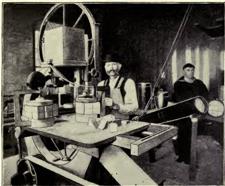
PLATE 3.—Shaping charges of gun-cotton with a band saw.
